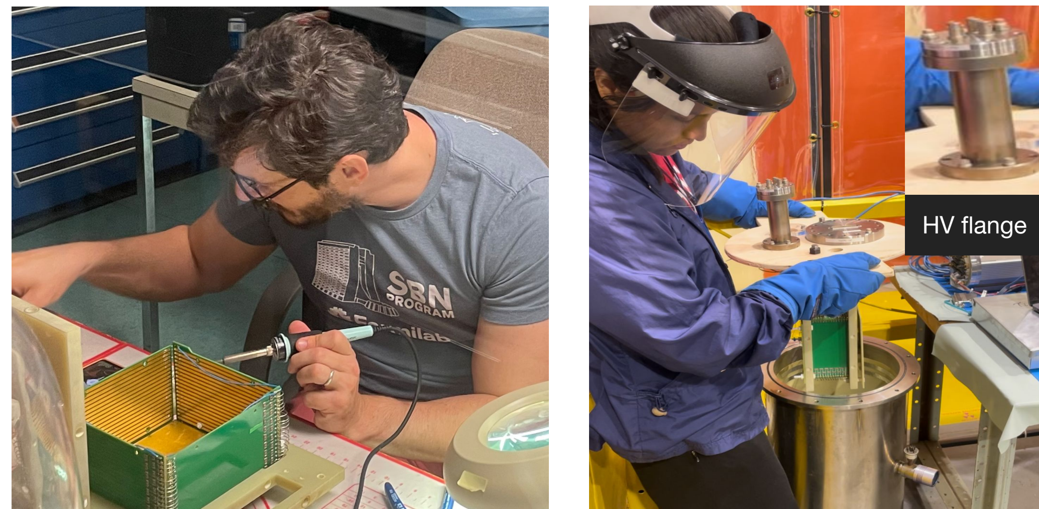
Fixing TPC resistors (left). Testing TinyTPC in dewar (right)
