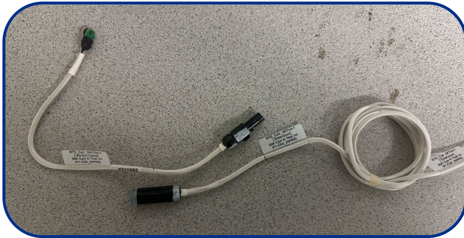
An RTD cable with an extension cable beside it. Labeling is shown.
