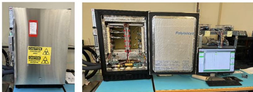
FIG. 5. Burnin box for module testing at Fermilab.
