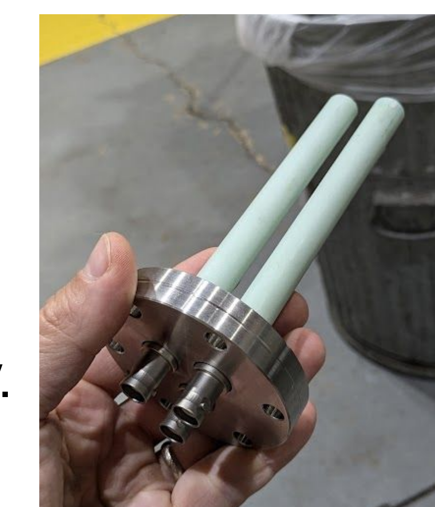
Old high voltage flange
