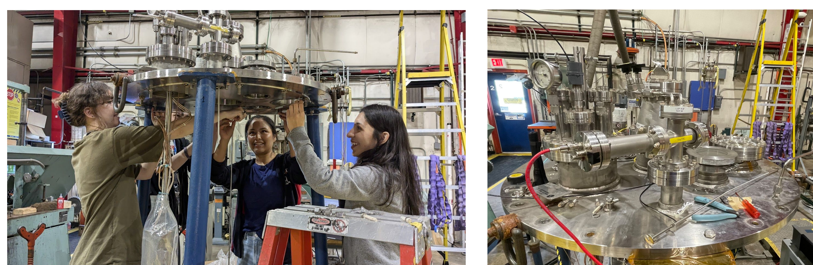
Performing tests on TinyTPC mounted to the cryostat (left), Top of cryostat lid (right)
