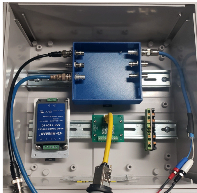
Figure 6. Electronics mounted inside the enclosure (Note: Not all wires attached, hole punch outs not yet made at this point.)
