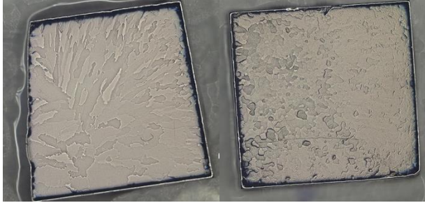
Illustration 1. Visible grain structure after polishing; HEAs 2.3 left and 2.7 right.
