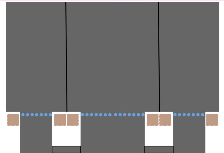
Wheels can live in the space between the coils – only the top edge has to be above the coil height
