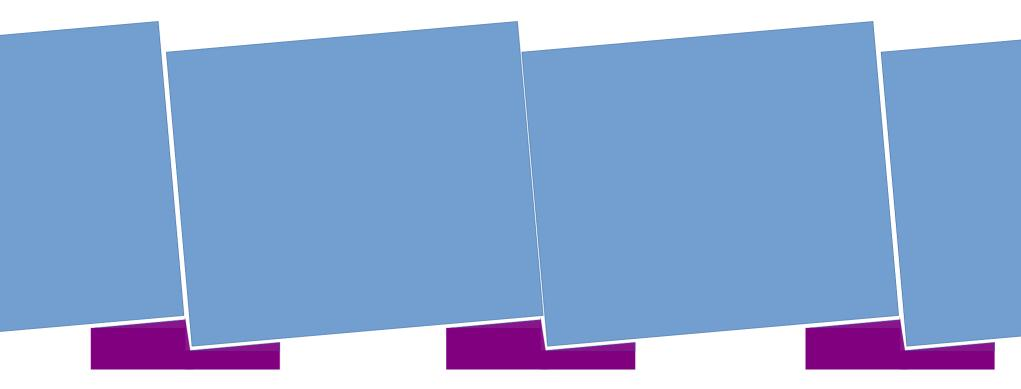
Modules have slight width variation due to scintillator tolerances Absorb these tolerances by not filling the whole triangle Assume aluminium for these
