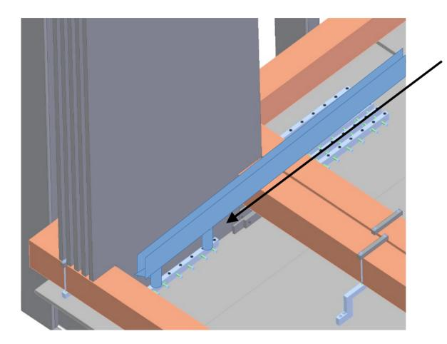
Ideally, integrate spacers with "legs" that a rail can be mounted on
