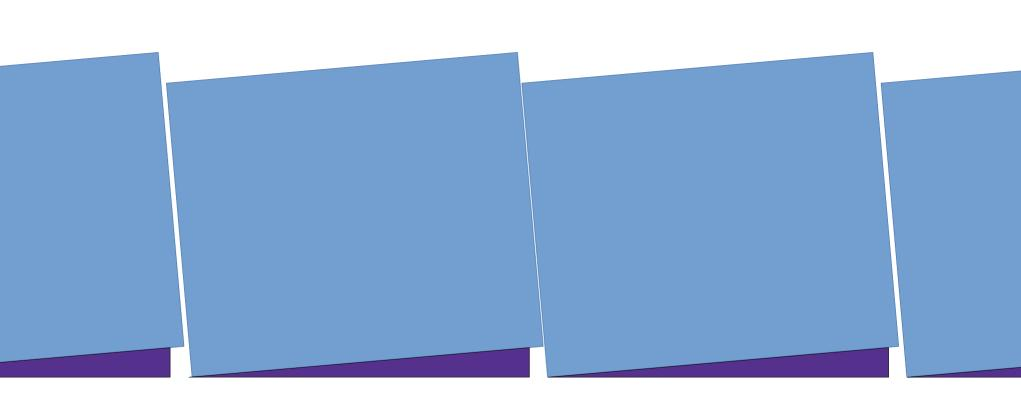
Modules have slight width variation due to scintillator tolerances Absorb these tolerances by not filling the whole triangle Assume aluminium for these
