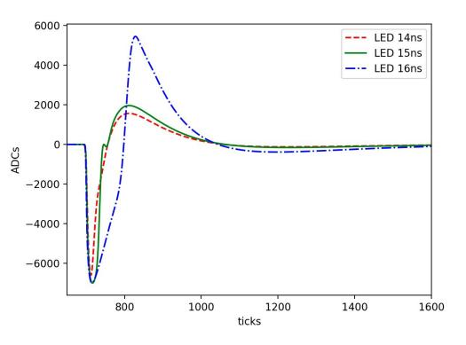
We observe saturation effects at 7000 ADC in DAPHNE (max VGAIN) (probably the cold amplifier board saturating).
