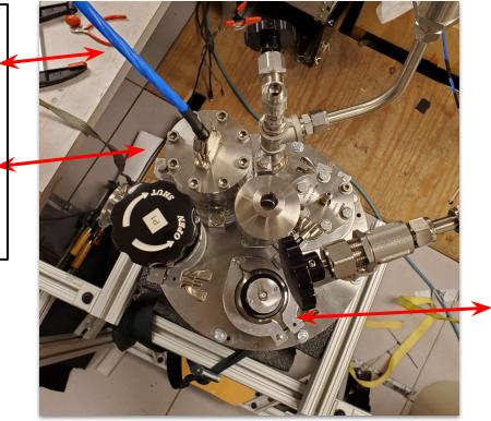
Shielded enclosure with LED and view port for LED tests
