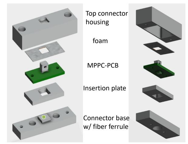
Shown is single channel connector w/o LED light injection Concept can be expanded to 8 channels w/ LED
