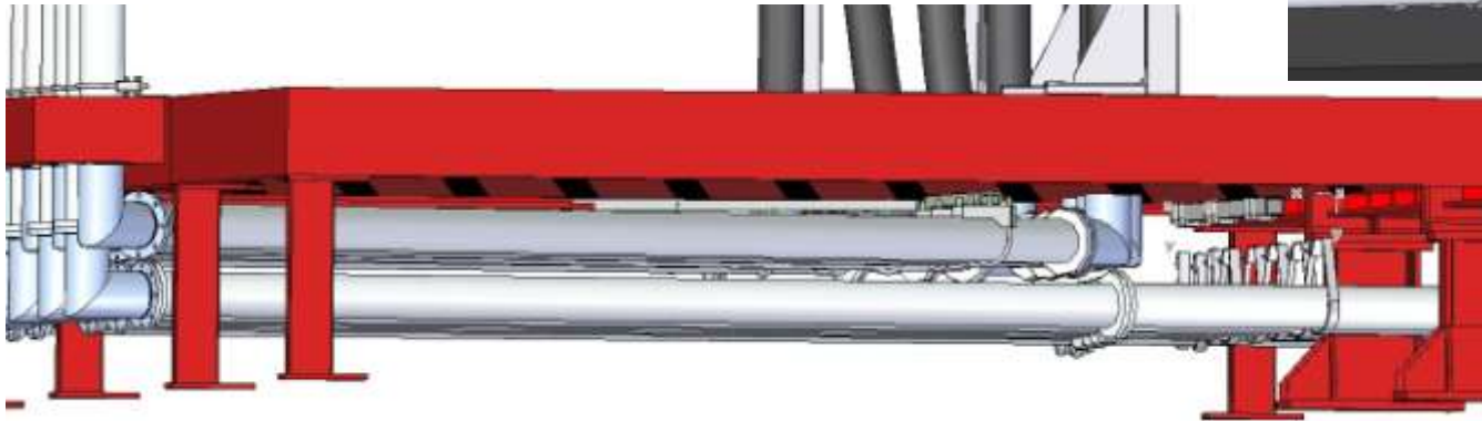
No support structure on floor. Clear access for cable trays and water pipes.
