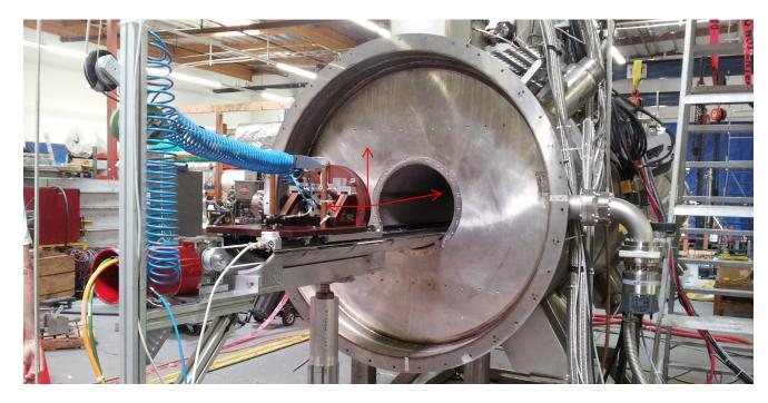
X axis along the magnet on direction opposite to beam direction
