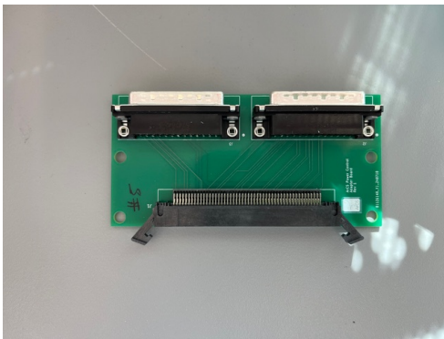
Fig. 14. Adaptor board from DB-25 cables to ribbon cables
