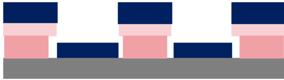
Undercut helps to 'break' the film
