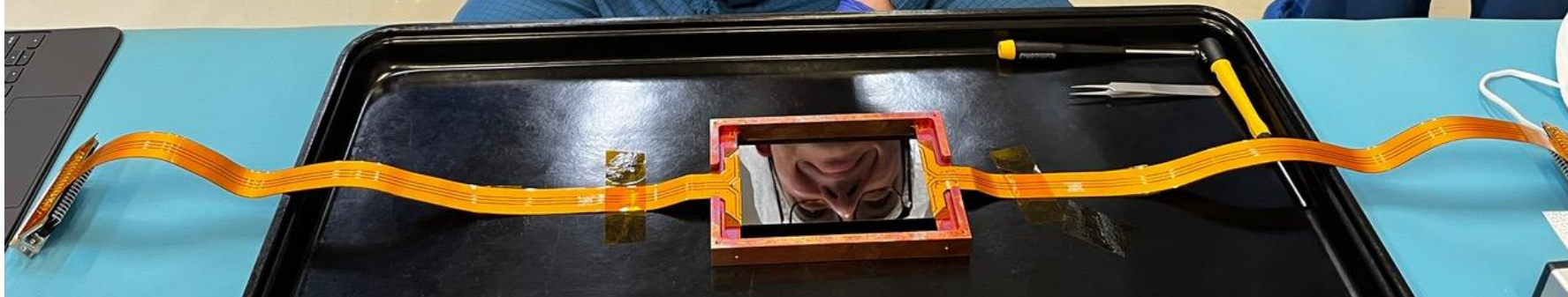
6k x 4k CCD for DAMIC@SNOLAB / Alvaro Chavarria (U Washington)
