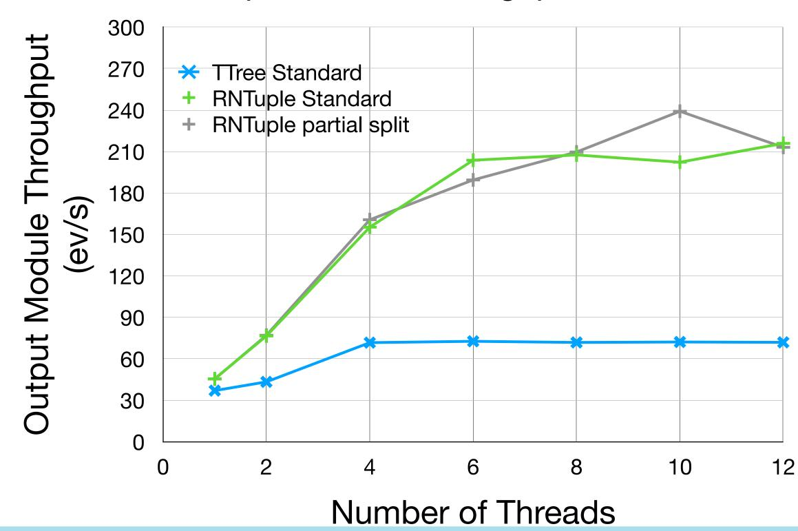
OutputModule Throughput vs Threads
