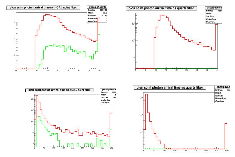
50 GeV incident particles Red is Cerenkov, green is scintillation. Lights scaled down after creation as Where "C" is crystal and "O" is other materials.
