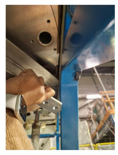
Drilled holes were not aligned with those on the flange
