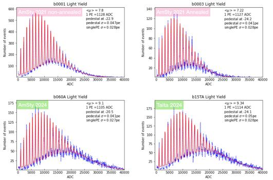
The light yield in photoelectron (PE) was estimated by fitting each light yield spectrum with a gaussian of each PE peak convoluted with a Poisson and Sr<sup>90</sup> energy spectrum. The first 10 peaks in each light yield spectrum were used to determine the spectrum's ADC-to-PE calibration.
