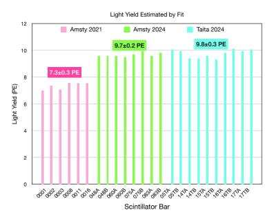
On the average, the observed light yields of new Amsty's bars and Taita's bar are about  $1.3\pm0.1$  times higher than those of the Amsty's 2021 bars, consistent with our simulation. All bars used in this study were co-extruded with TiO<sub>2</sub> reflector.
