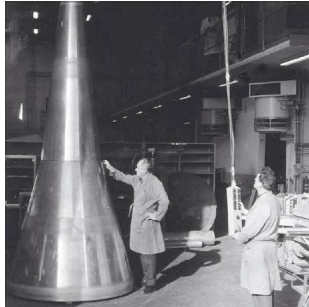
An inner conductor for the new neutrino "reflector". CERN Courier Archive
