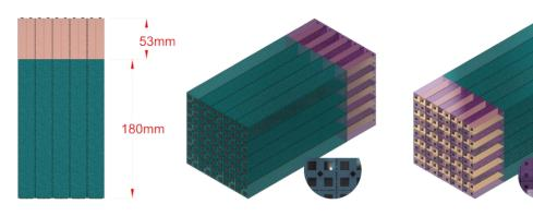
22±0.1 x 22±0.1 Large cell size =  $\sim$ 22.3 x 22.3 (tolerance of xtal size + carbon fiber srtruct)
