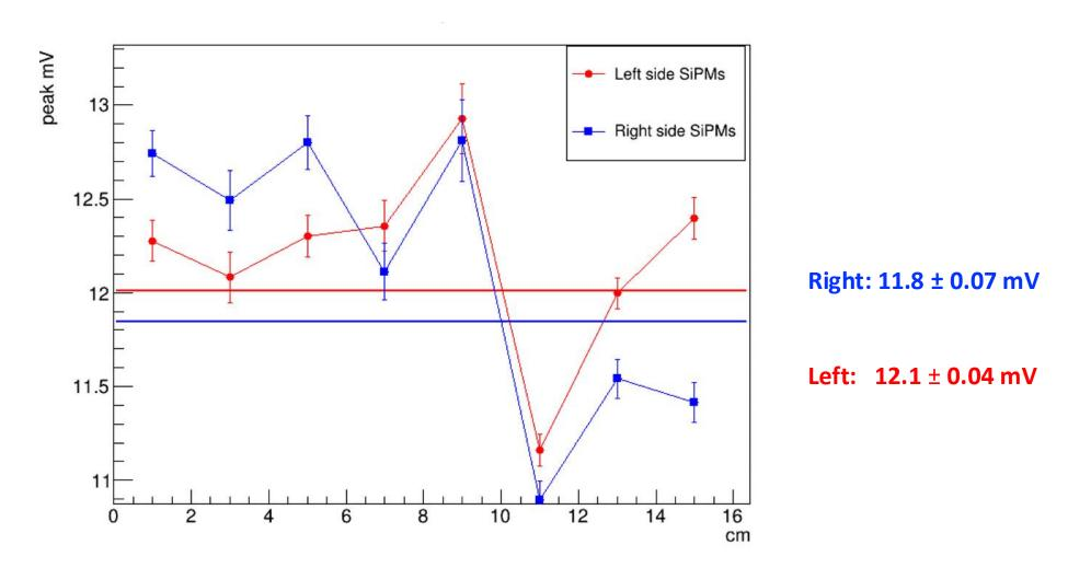
Elgin silicone cookie left side, *Dowsil optical coupling grease* right side of the crystal. Run 245
