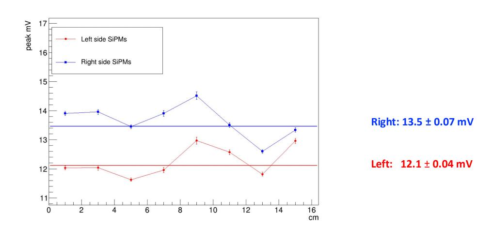
Elgin silicone cookie left side, *Dowsil optical coupling grease* right side of the crystal. Run 244
