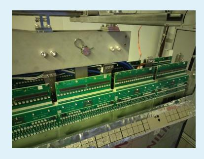
These leakage current tests are important, as we cannot risk frying the cold electronics through a problematic board drawing a large current
