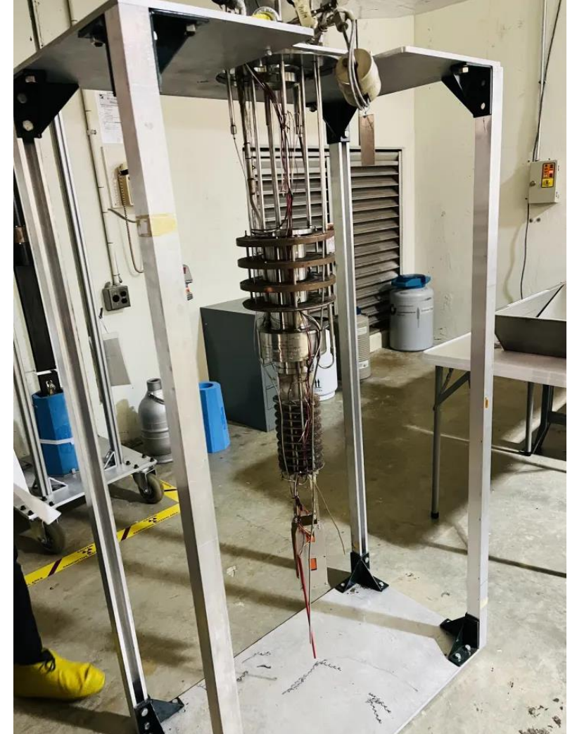
Refrigerator: Installation of temperature sensors
