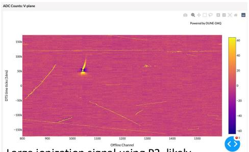
Large ionization signal using P2, likely happening right outside the field cage. No through-going track.
