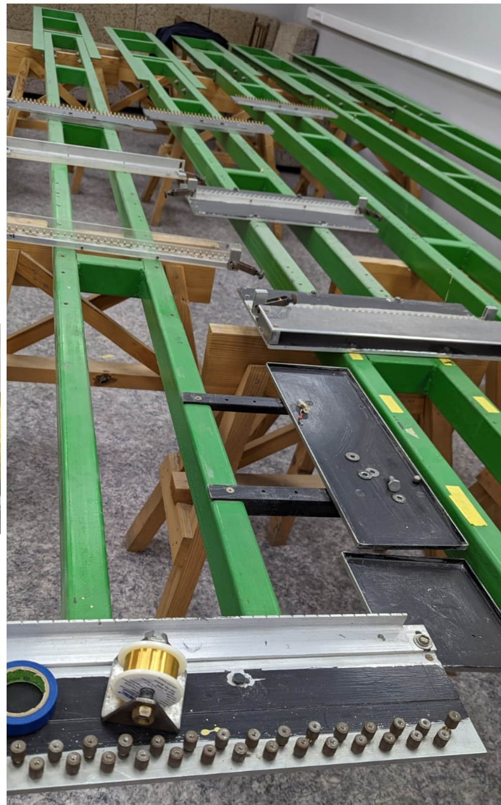
MA tooling developed for COMPASS to glue spacers on 4m long wires before insertion into straws
