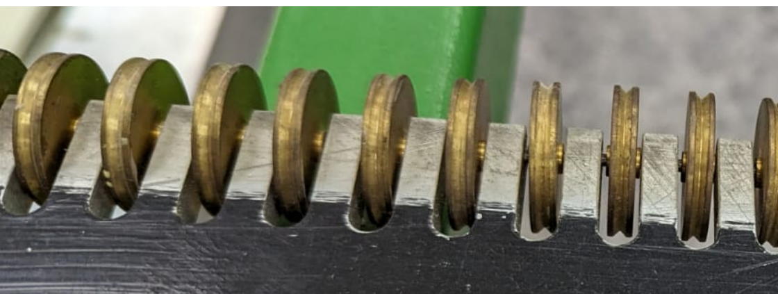
MA tooling developed for COMPASS to glue spacers on 4m long wires before insertion into straws
