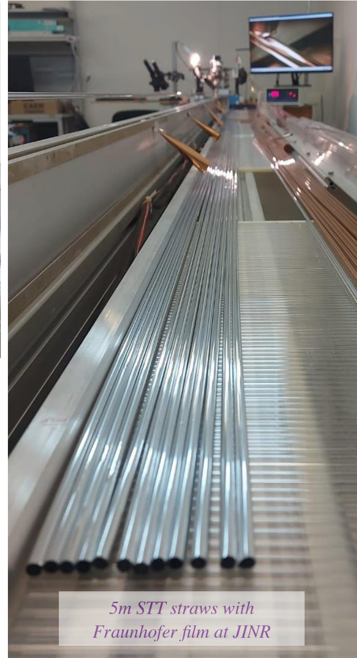
Straw production unit (5m) at JINR
