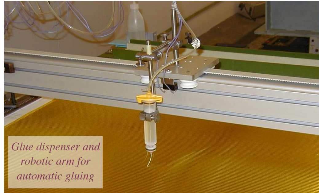
Assembly table for 4m modules
