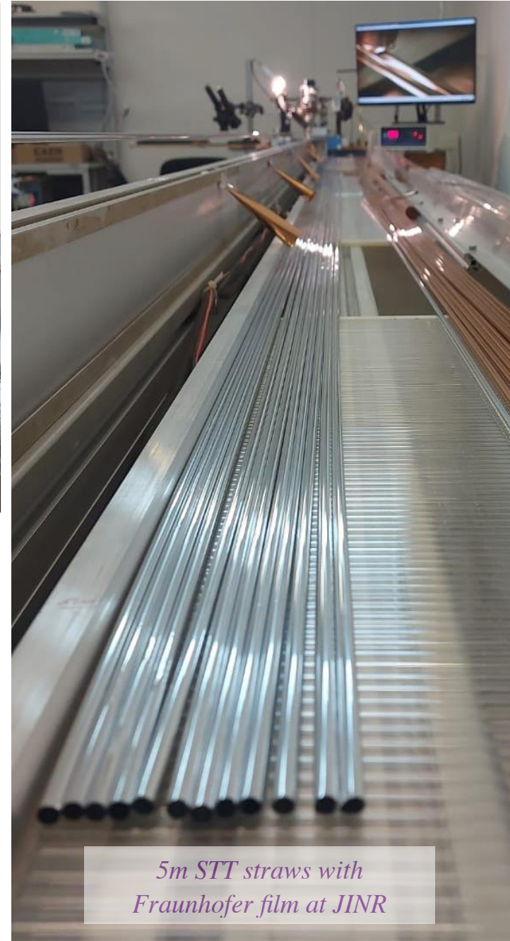
Straw production unit (5m) at JINR
