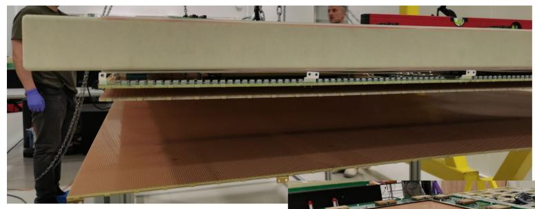
Previously, anodes were replaced with FEMBs still installed. But the bias lines were connected and terminated.
