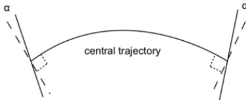
Figure 6-1. Edge angle in a magnet
