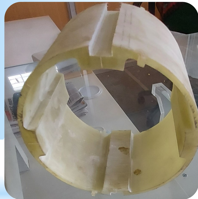
G-10 corrector coil positioning cage
