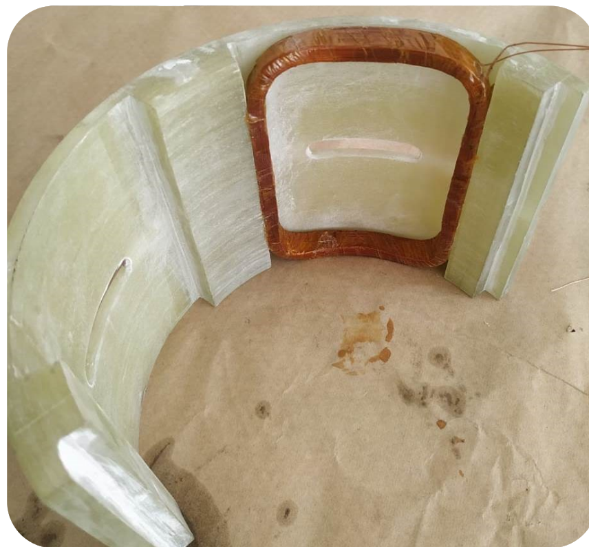
Corrector coil positioned inside cage
