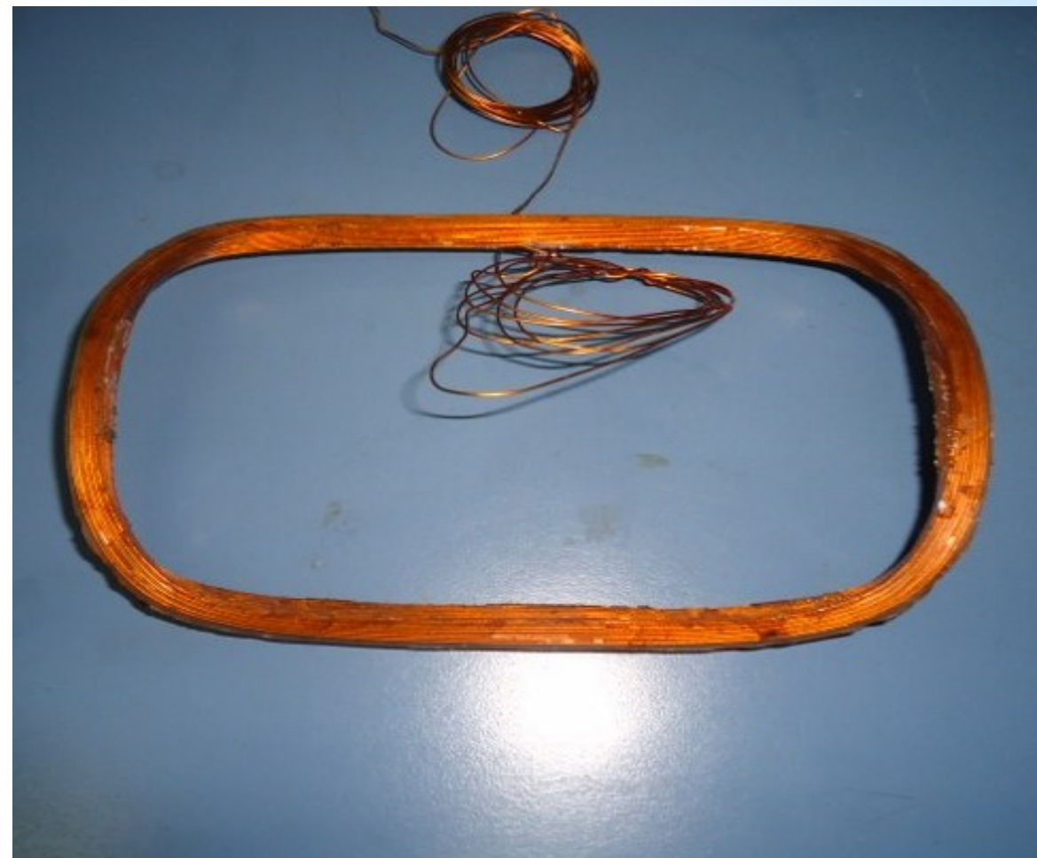
Corrector coils after winding
