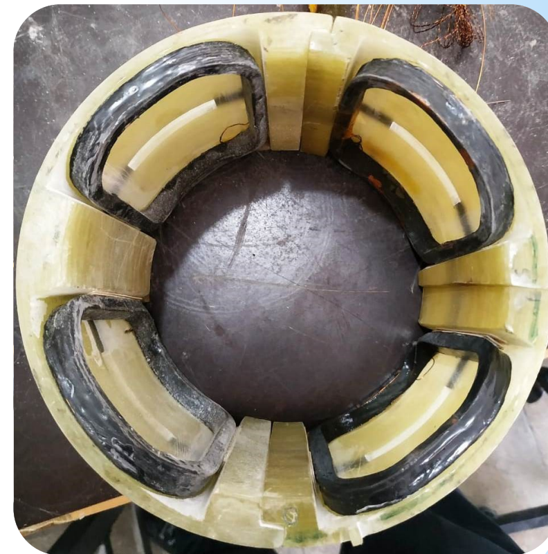
Corrector coil positioned inside cage
