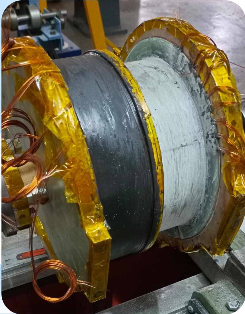
Bucking coil 1 last layer after STYCAST
