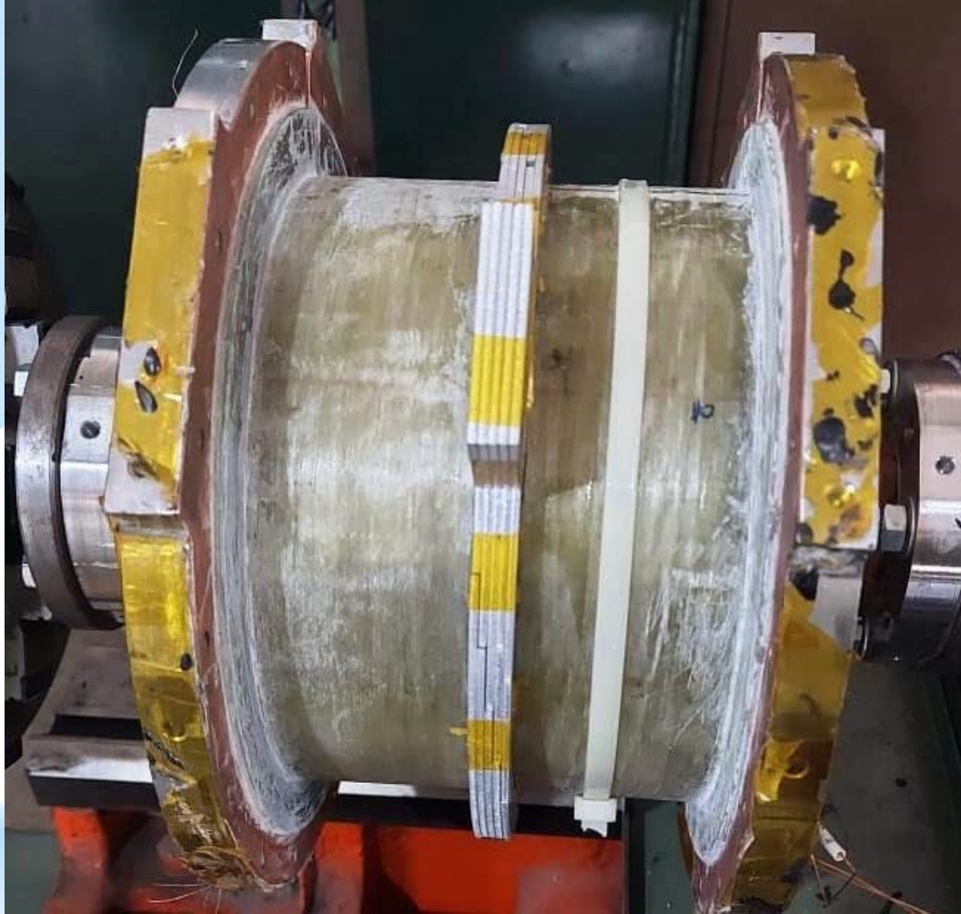
Surface before bucking coil winding
