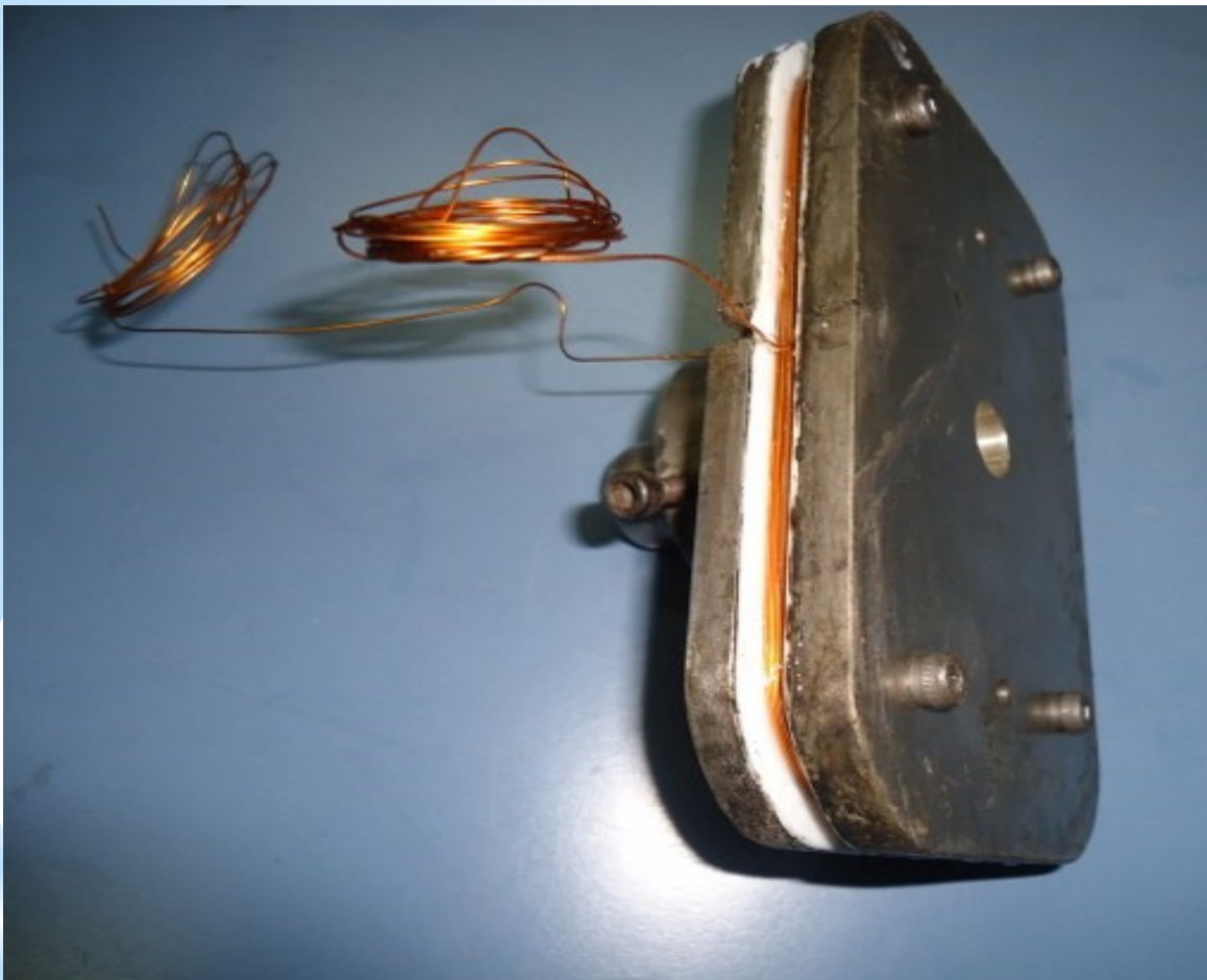
Core insulation with Kapton
