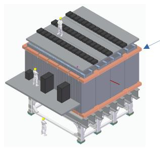
Depending on how much the fringe field affects the performance of the CAEN 5202 FEBs will determine the final length of the signal cables and how high the EB mounting platform will need to be placed above the surface of the TMS
