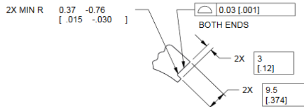
3.12: Yoke 3mm x 9.5mm gap key grooves.
