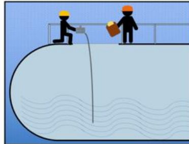
Hydrogen Sulfide (H 2 S) (Slightly heavier than air)
