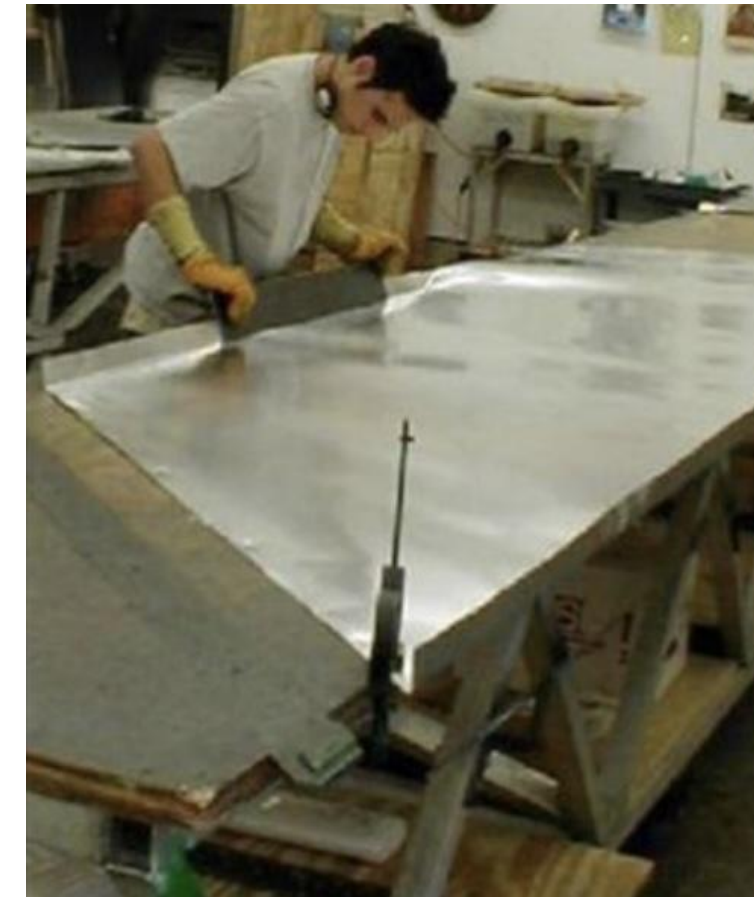
MINOS bottom case cutting and flange forming
