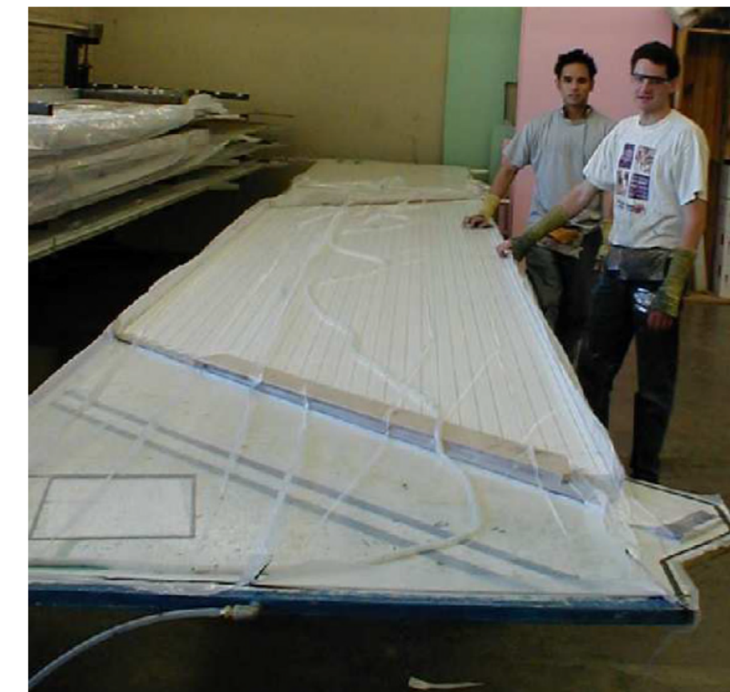
MINOS bottom case vacuum bonding
