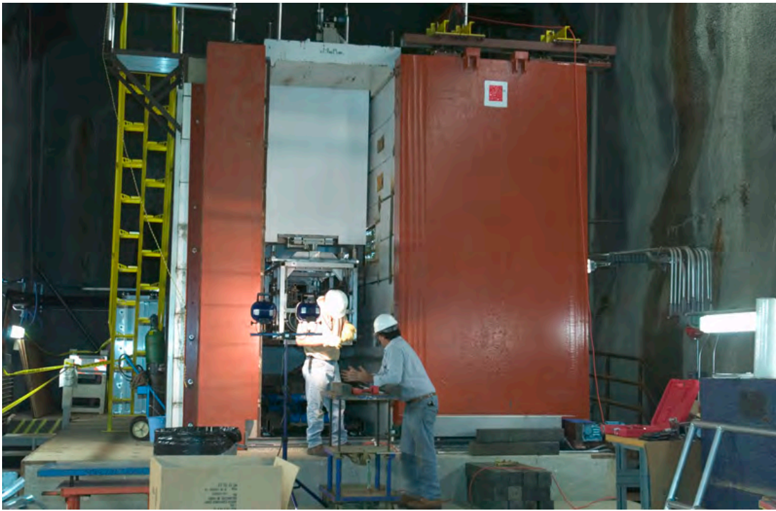
Figure 22: NuMI Workcell for hot handling operations and failed component replacement. Image shows NuMI target module in the workcell for a hot handling procedure dry run during NuMI construction
