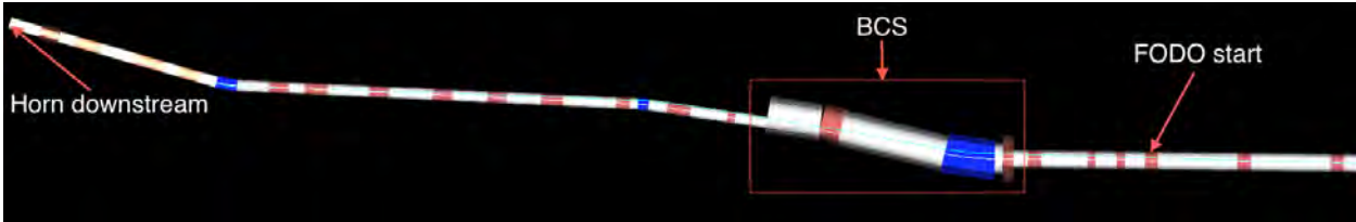
Figure 40: The optics of \pi transport and injection. The optics shown start in the decay straight and end at the downstream end of the horn (left to right).larger
