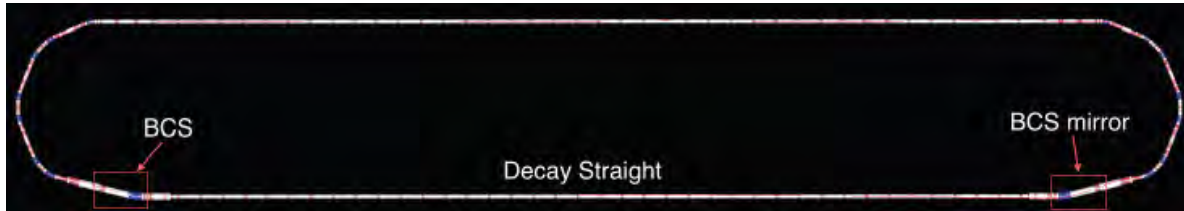
Figure 43: Racetrack ring layout. Pions are injected into the ring at the Beam Combination Section (BCS). Similarly, extraction of pions and muons at the end of the production straight is done using a mirror image of the BCS.
