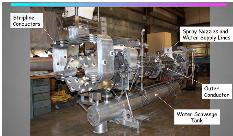
Figure 32: NuMI Horn 1 ready spare.
