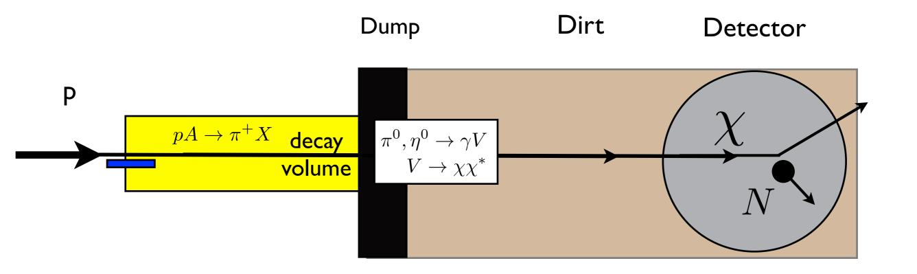
Optimally, dump should be positioned immediately following beam line
