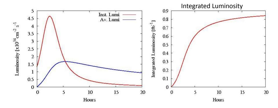
Peak Luminosity =  $4.6 \times 10^{34} \text{ cm}^{-2} \text{ s}^{-1}$ Optimal store time ~ 6 hours Integrated luminosity over a 10 hr store ~  $0.8 \text{ fb}^{-1}$
