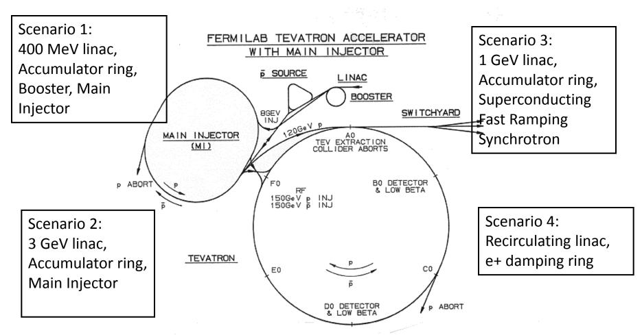
Figure 1-2. Schematic View of the Main Injector Connections to the Booster, Antiproton Source, Tevatron and Switchyard.
