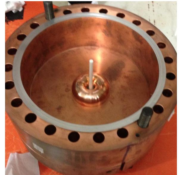
Frequency = 814.544 MHz @ 1 atm Q_L = 4,250 from RF calibration
