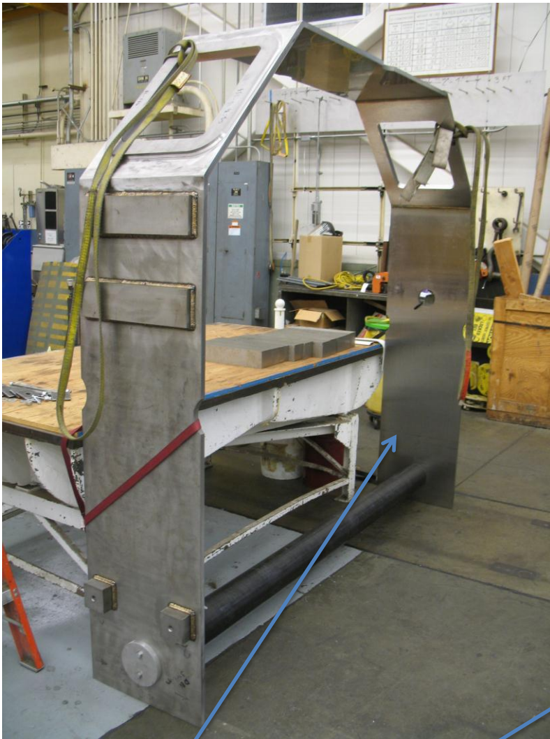
CC Cryostat Vessel Fabrication at LBNL
