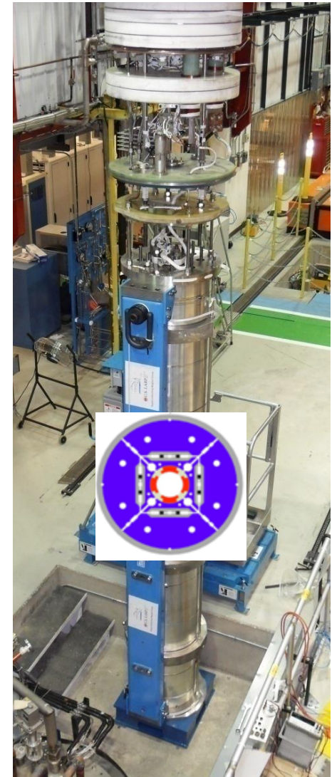
4-m long Racetrack, D and Q mirror configurations; 90-mm quadrupoles
