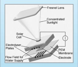
Advantages: Operational system has already been demonstrated with 18% efficiency.<sup>1</sup>
