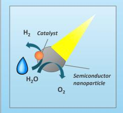
Advantages: Offers a simple architecture with the potential for low materials cost.
