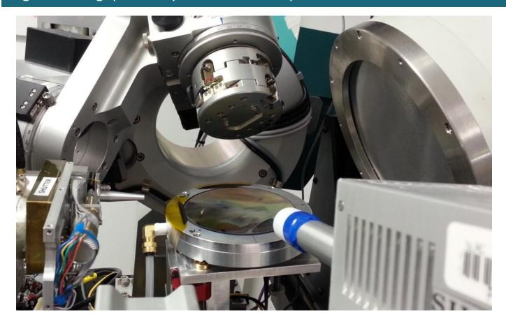
Current setup: 1,000-2,000 samples/day x10 flux -> 10,000 samples/day Faster detector -> 100,000 samples/day May become motor speed limited
