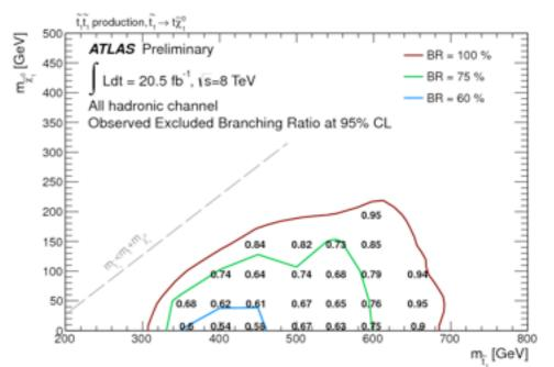
Stop masses between 320 and 660 GeV are excluded at 95% CL for a nearly massless LSP (BR=100%).
