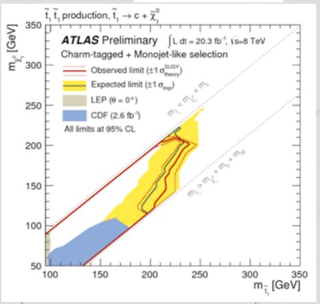
Stop mass of 200 GeV is excluded at 95% CL for m(Stop)-m(LSP) < 85 GeV.
