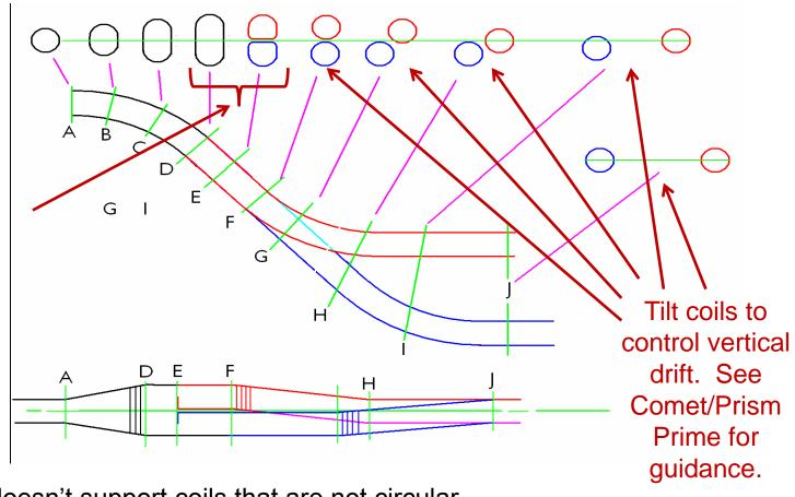
G4beamline doesn't support coils that are not circular.
