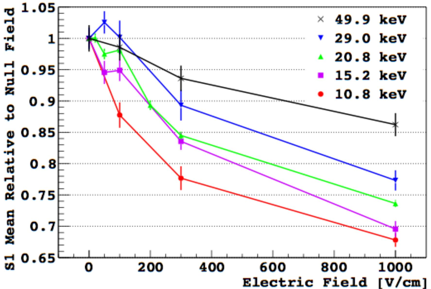
Past and current estimates of sensitivity for noble liquid TPC dark matter searches assume the light yield for nuclear recoils is only slightly affected by the presence of a drift field
