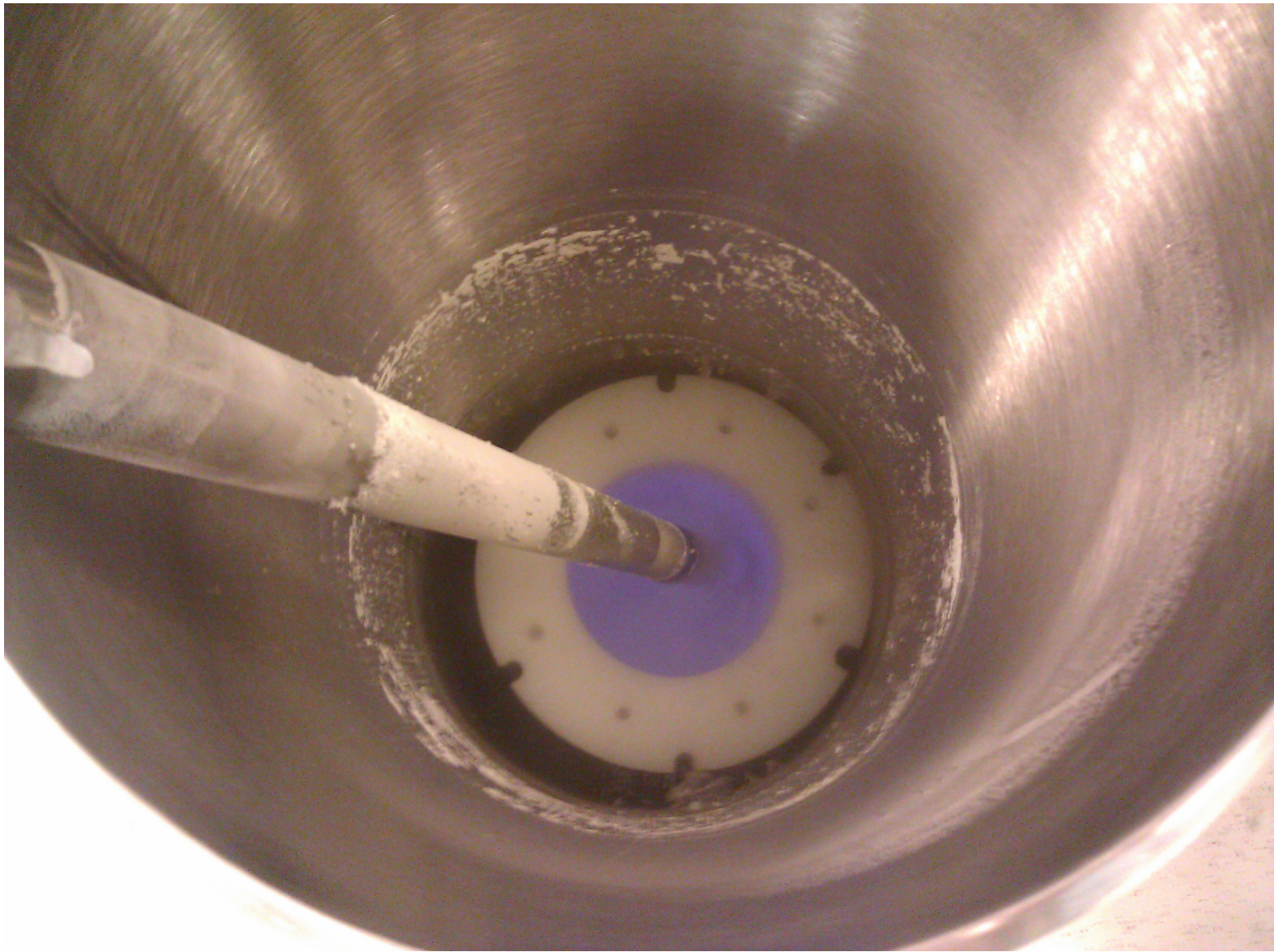
Glowing PE after Continues Breakdown in Liquid Argon During destructive test!
