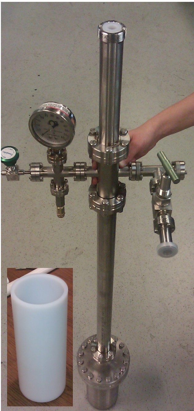
Setup to test FT at real working temperature and pressure
