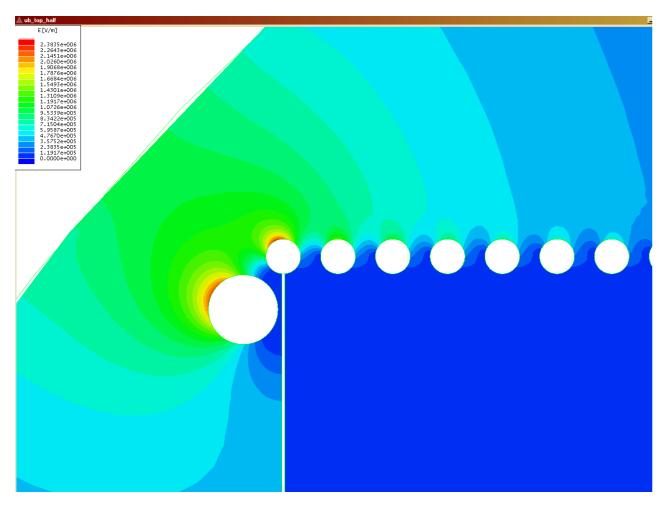
Simulation near point(s) of closest approach max  $E \rightarrow 24$  kV/cm @ HV=125kV
