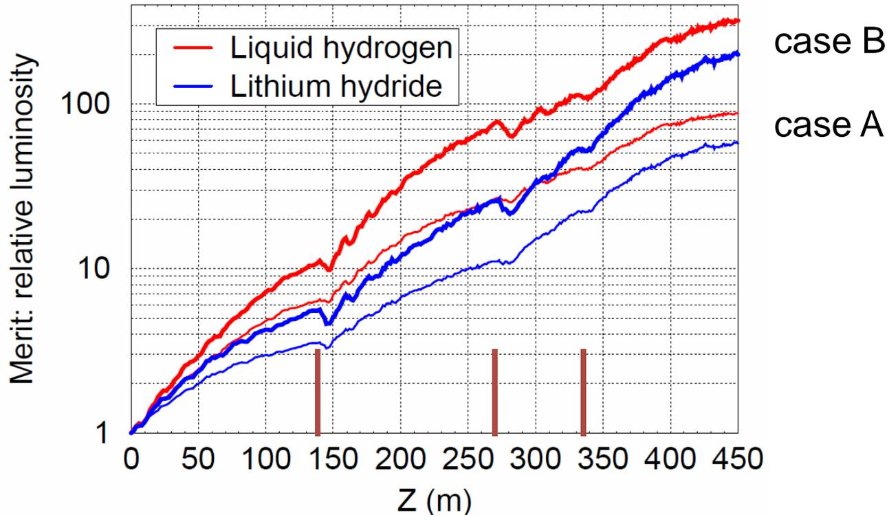
Higher merit in case **B** does not mean a higher luminosity but it means higher sensitivity of the luminosity to the beam emittance.
