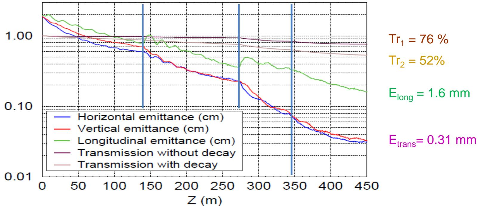
Emittance of the cooled beam is actually the same as before the replacement but transmission has fallen:  $90\% \rightarrow 76\%$  without decay, and  $62\% \rightarrow 52\%$  with decay.
