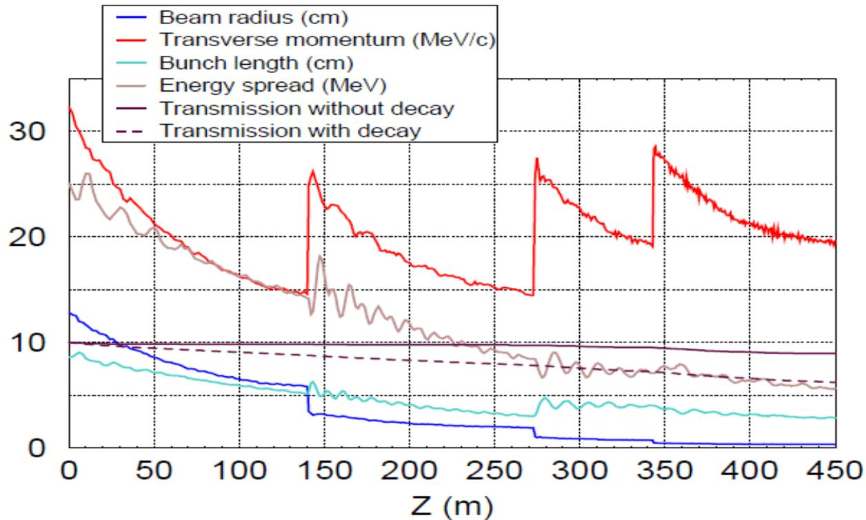
The beam transverse momentum steeply rises between the stages. It causes a perturbation of the beam energy spread (correlations!) and results in increase the longitudinal emittance.
