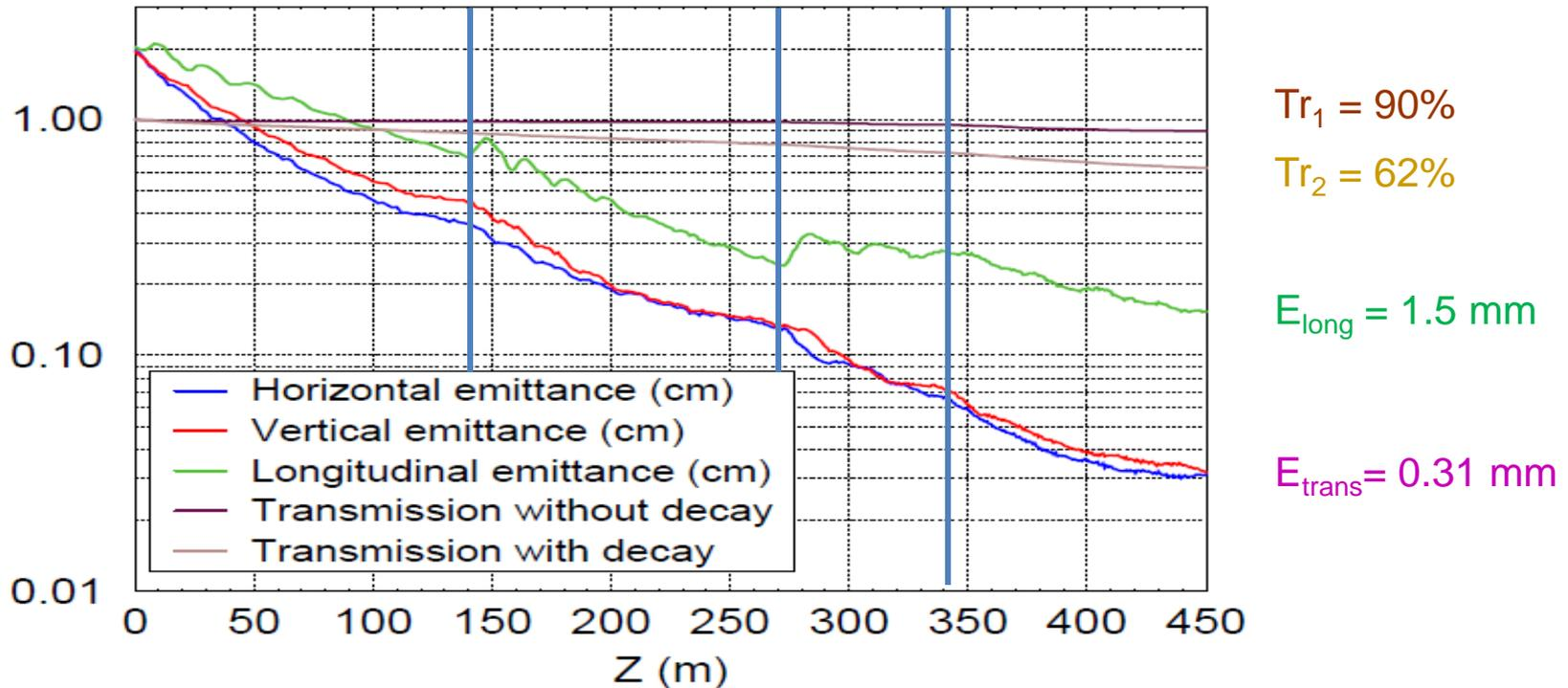
Longitudinal emittance increases at the transition from each stage to next one.
