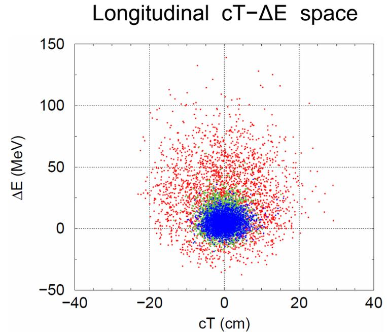
Red – injected beam, green – after 2<sup>nd</sup> stage, blue – at the end of the channel.
