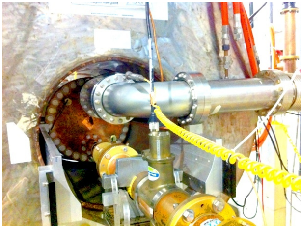
HPRF cavity in Lab G solenoid. Coaxial input coupler and vacuum lines are also shown.
