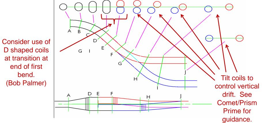
G4beamline doesn't support coils that are not circular.
