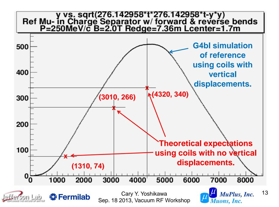
In analyzing the effect of a charge splitter, we prefer to have a configuration that has an analytic description against which we can validate our simulations.
