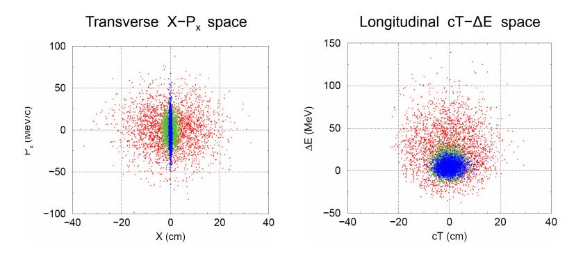
Red – injected beam, green – after 2<sup>nd</sup> stage, blue – at the end of the channel.
