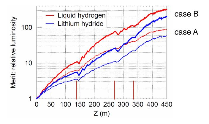
Higher merit in case B does not mean a higher luminosity but it means higher sensitivity of the luminosity to the beam emittance.
