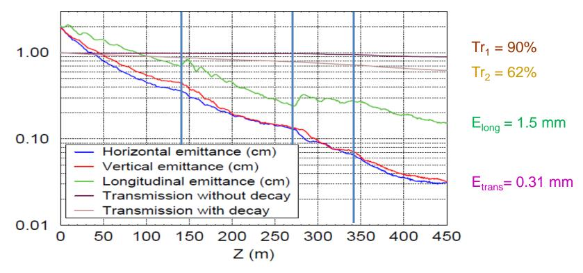
Longitudinal emittance increases at the transition from each stage to next one. The effect is caused by longitudinal – transverse correlations (nonlinear) which cannot be controlled and corrected by the (linear) matching sections.
