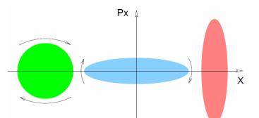
Single 90° cell would require magnetic field up to 20 T Single 270° cell would require a modest field but creates unacceptable chromatiity. Cooling with self-consistent initial distribution, and matching section or matrices between the stages 1<sup>st</sup> and 2<sup>nd</sup> stages with LH<sub>2</sub> absorbers, 3<sup>rd</sup> and 4<sup>th</sup> – with LiH
