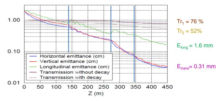
Emittance of the cooled beam is actually the same as before the replacement but transmission has fallen:  $90\% \rightarrow 76\%$  without decay, and  $62\% \rightarrow 52\%$  with decay.
