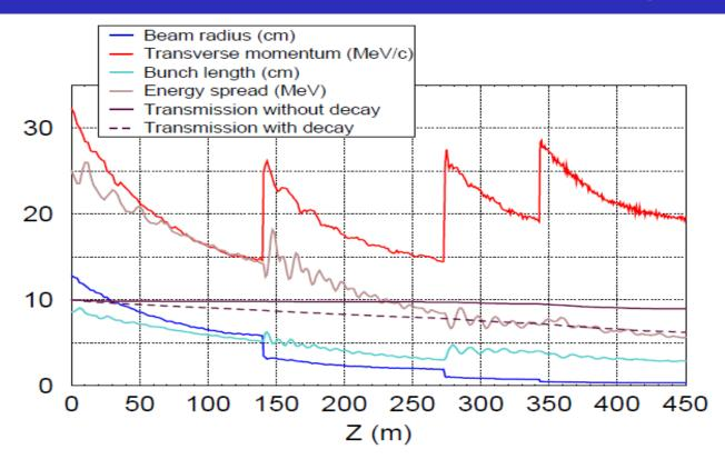
The beam transverse momentum steeply rises between the stages.
